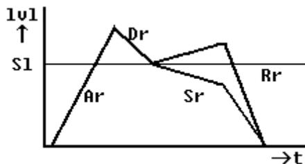
**Ar** Attack rate, which specifies the speed at which the volume increases from zero to it's maximum value, as soon as the note on is given. The slope can be set to linear or exponential.
